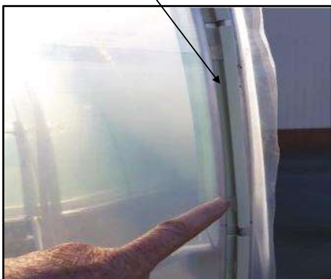
(Pic L1): Use the 200mm inserts only on front face of the curved part at each end
