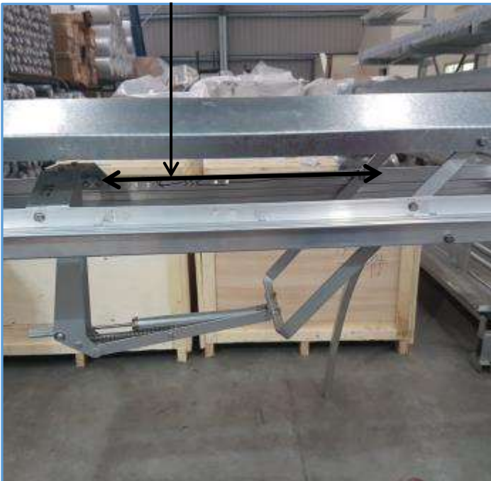
437mm from handle pivot bolt to first bracket bolt (457mm to 2 nd bracket bolt)
