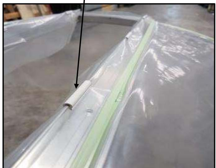
END AND LOUVRE END WALL COVERS – use the Lockstrip holding system for the hoop and end wall stud parts and Duralock 2 holding system for the base rail part.
