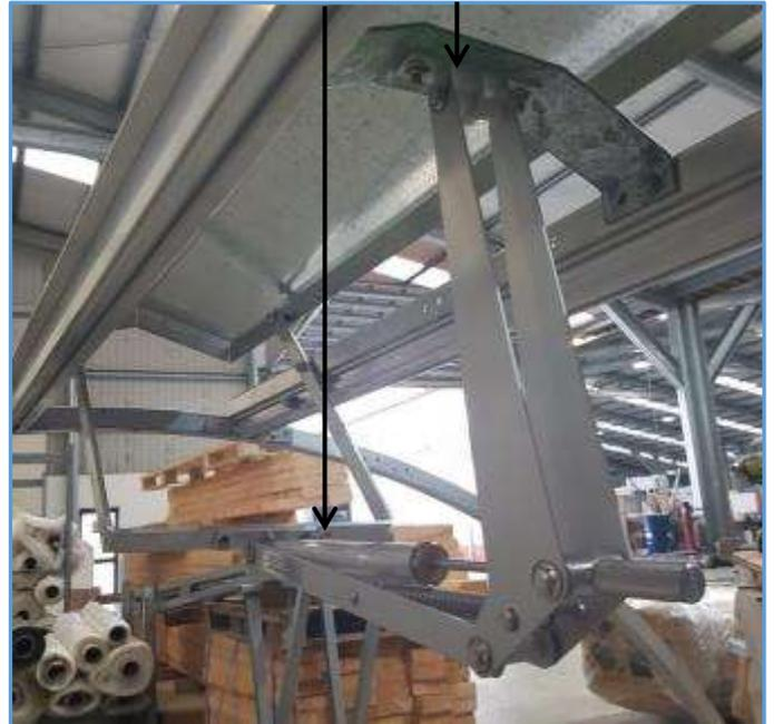
437mm from handle pivot bolt to first bracket bolt (457mm to 2nd bracket bolt)
